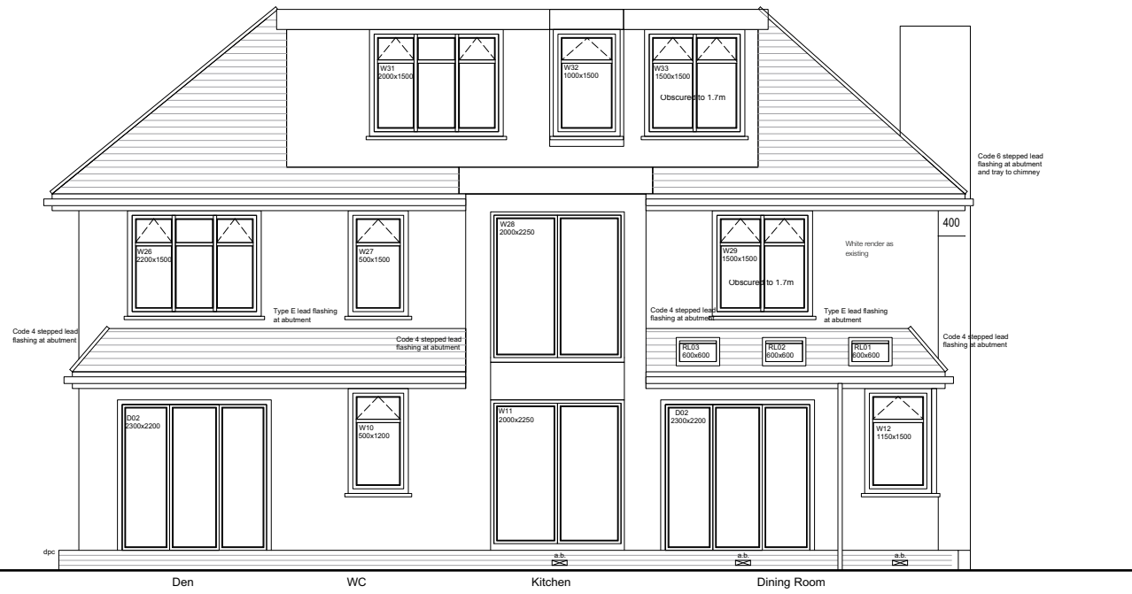
West Elevation [Rear] 1:50
